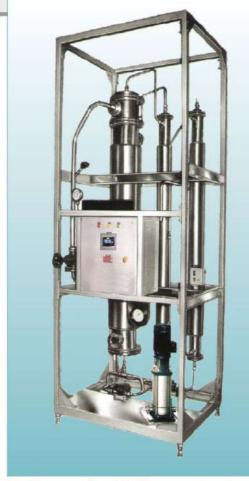
Ideal for generation of sterile pyrogen free steam used in the steam sterilizers and for SIP of vessels, pipelines, lyophilizers, etc.
